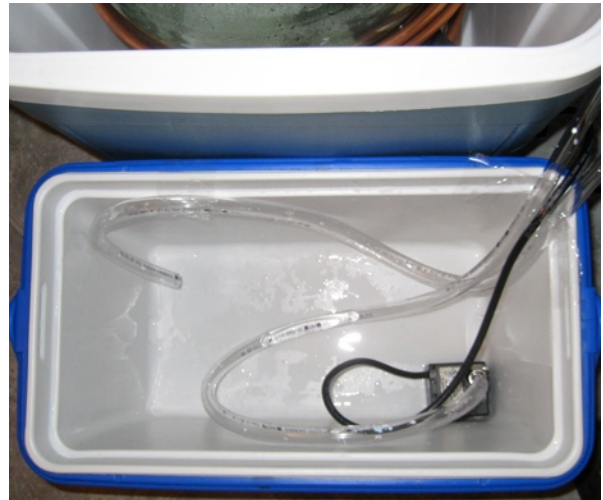
Figure 3. Pump assembly in second cooler.
