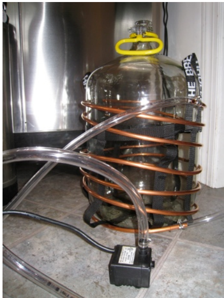
Figure 1. Copper coil wrapped around carboy and attached to pond pump with vinyl hose.
