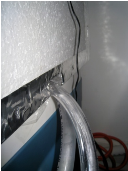
Figure 2. Notch through foam lid for vinyl tubing.
