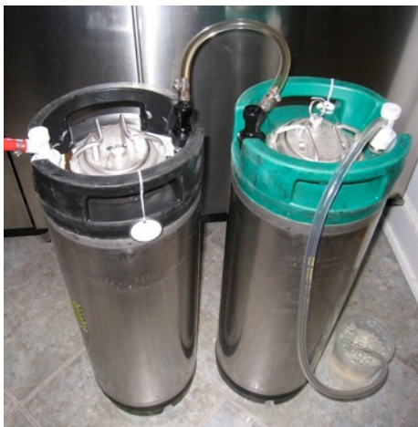
Picture 5. Setup to transfer from secondary fermenter to final keg.
