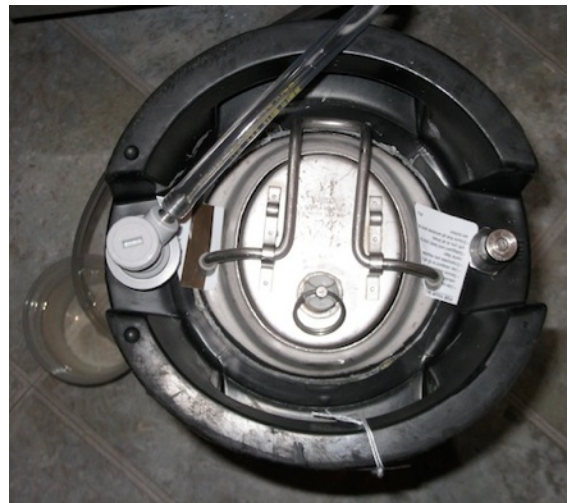
Picture 4. Place plastic shims under lid lock feet to ensure a tight seal.
