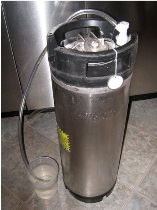
Picture 3. Blow-off hose attached to gas in port.
