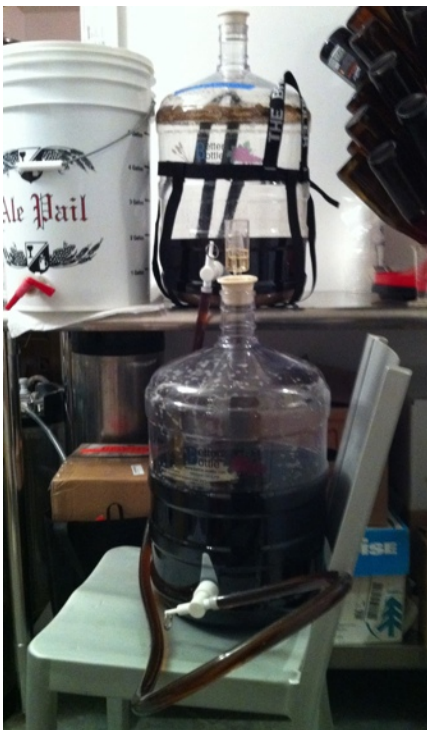
Picture 4: Racking brown ale between two BetterBottles® using 1/2 ID vinyl hose, SimpleFlo™ valves and racking adapters
