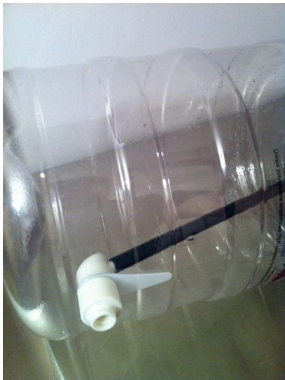
Picture 5: Using racking outlet install rod to assemble racking adapter in bottle
