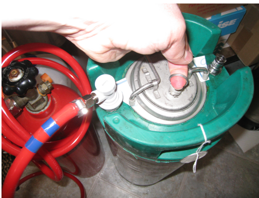
Photo 3: Purge the keg using CO 2 . Be sure to vent any residual pressure from the keg before proceeding to the next step.
