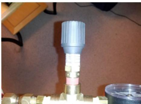
4. Set the relief valve using the regulator on your CO<sub>2</sub> tank.
