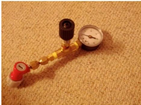
Spunding valves are used in commercial breweries on bright tanks to allow pressure to rise naturally to a certain level. By using an adjustable pressure relief valve, the gas produced during fermentation can be used to naturally carbonate the beer to the desired level. Building a spunding valve for use on corny kegs is a quick and easy project that can be built in about 10 minutes.
