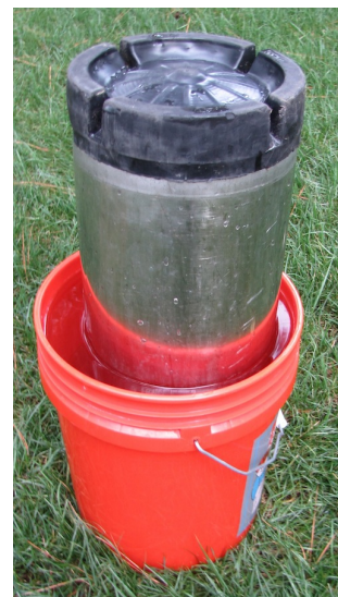
Soaking the keg upside in PBW to make sure the top comes clean too!
