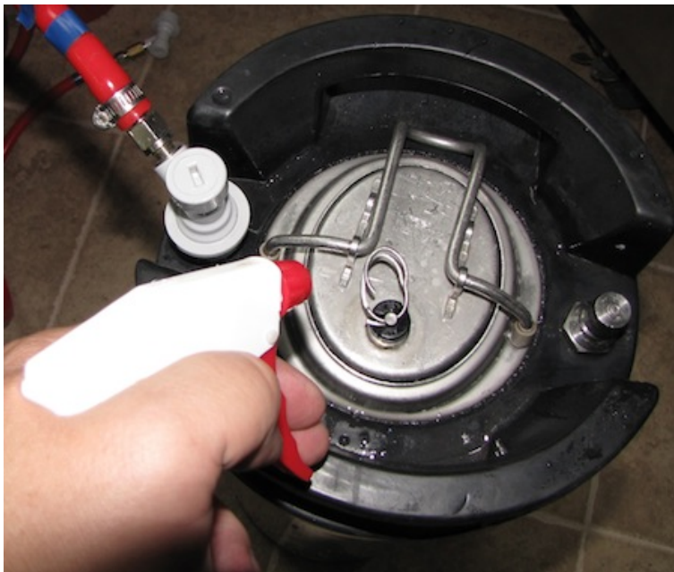
Leak check the keg and tighten any loose fittings. Spraying a little StarSan on the keg and looking for bubbles works well.
